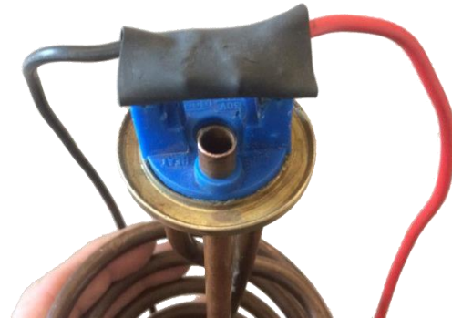
Figure 2.4 Element adapter fitted to flange-type element
