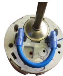
Figure 2.2 Bridging wire fitted to TSE Thermostat
